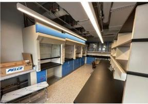
The newly renovated laboratory space for the Radiochemistry Faculty at Hunter College is comprised of two laboratories. One lab is for Radiochemistry, shown in this picture, with four fume hoods, a glove box and lab benches and cabinets/shelving for storage. There are lab services available. This space can be customized for the faculty member's research.
